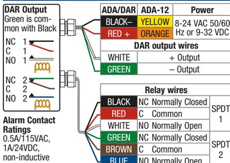
The ADA 2-conductor cable or the DAR 4-conductor cable with the RED and BLACK leads is for the gauge power supply. ADA models with the 12 foot lead option use an 8 conductor cable with YELLOW and ORANGE power leads.
